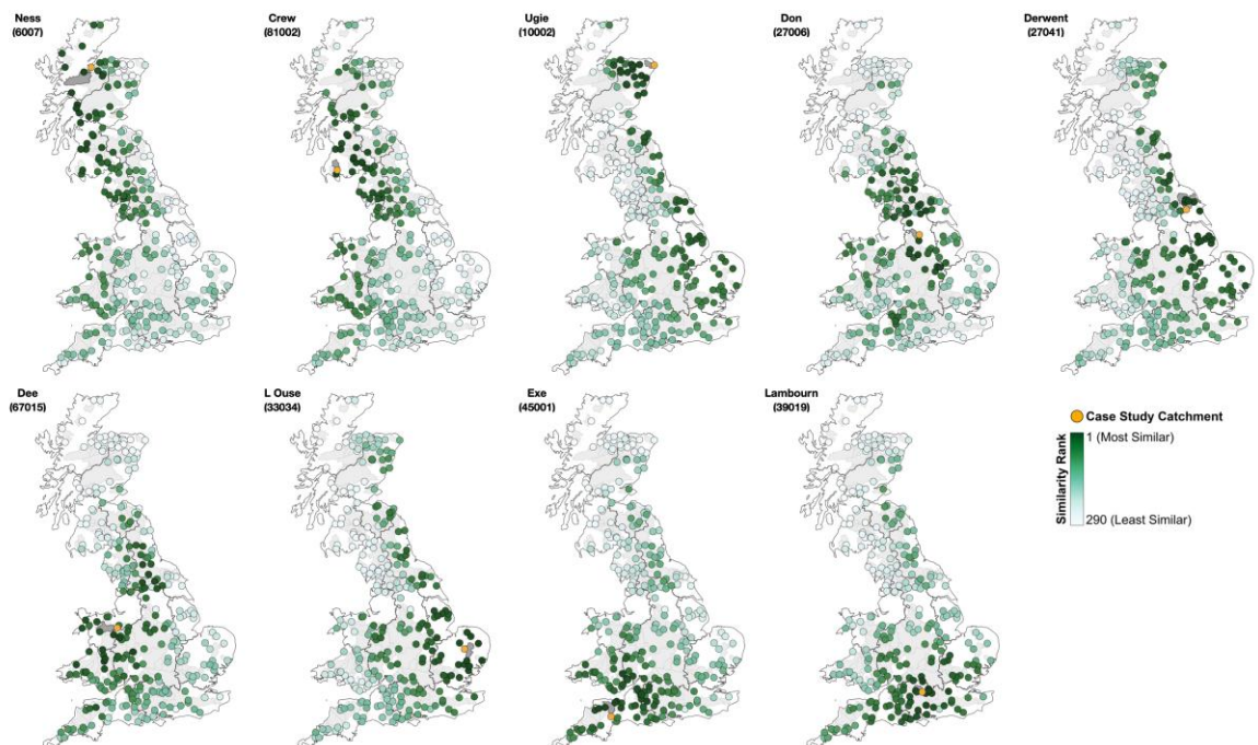
Figure 5: Similarity analysis results based on the NAO/EA SPI-1 correlation time series mapped in Figures 2 and 3. The case study catchment is highlighted in yellow. Catchments with lower values indicate those which have greater similarity in their NAO/EA monthly correlations to those of the case study catchment. Catchments with higher values indicate those which have NAO/EA correlations which are less similar.
