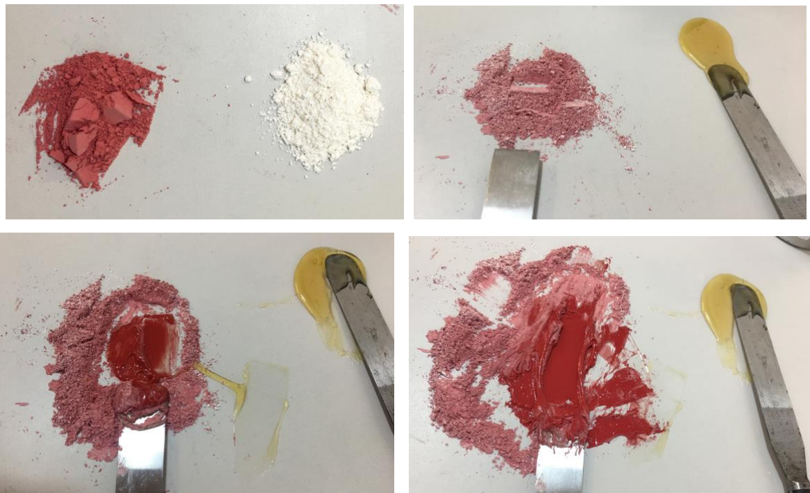
Fig.198. Four views of ink mixing. The dry components, colour and flux were mixed with the oil slowly
