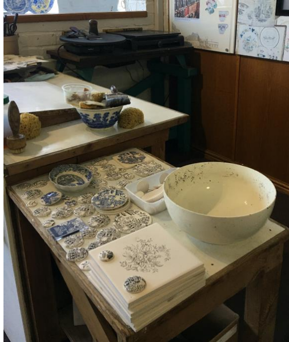
Fig. 66. The printed pieces are dried and ready to have a harden on firing, to remove printing chemicals and allow for a further glaze firing
