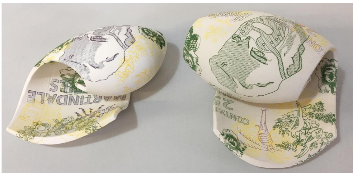
Fig.253. Tissue transfer method enables the print to adhere to intricate interior spaces, as once the printed tissue hits the ceramic surface it is permanent and remains firmly in place. This would be difficult to achieve with other forms of transfer printing
