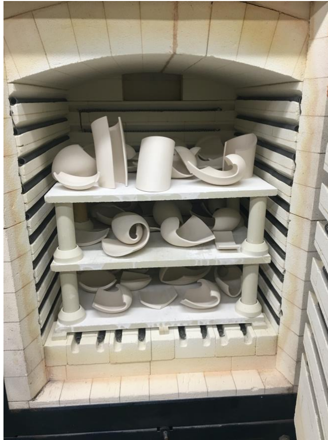
Fig. 193. The ceramic shapes after the biscuit firing at 1000°C.
