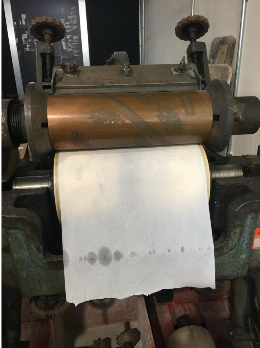
Fig.77. Redundant Pottery Printing Machine represents how the print is positioned in between two rollers, the upper one being the engraved roller. The engraved roller is attached to the machine with heated elements running through the core to warm the ink as it works itself into the pattern.
