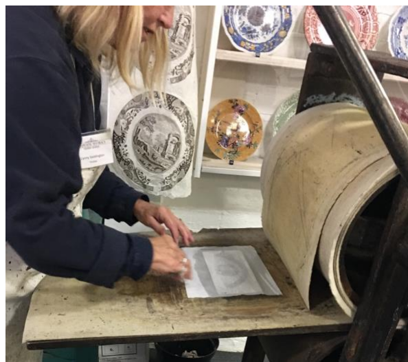
Fig. 61. The tissue is painted with a thin layer of size and placed face down onto the inked plate
