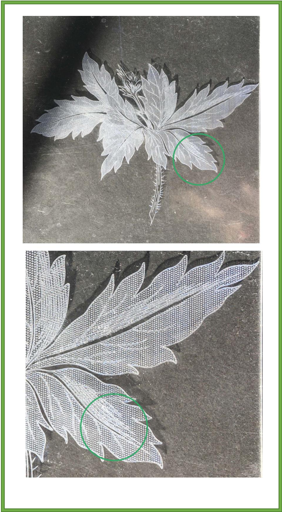
The laser engraved plate highlighted a more open dot mark, created with a pattern switch tool
