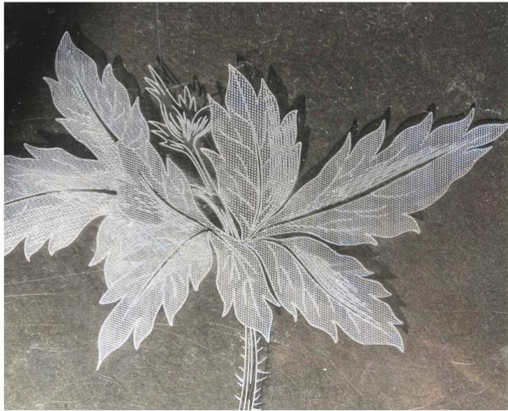
Illustrator image laser engraved (same variable form previous test) onto clear acrylic substrate
