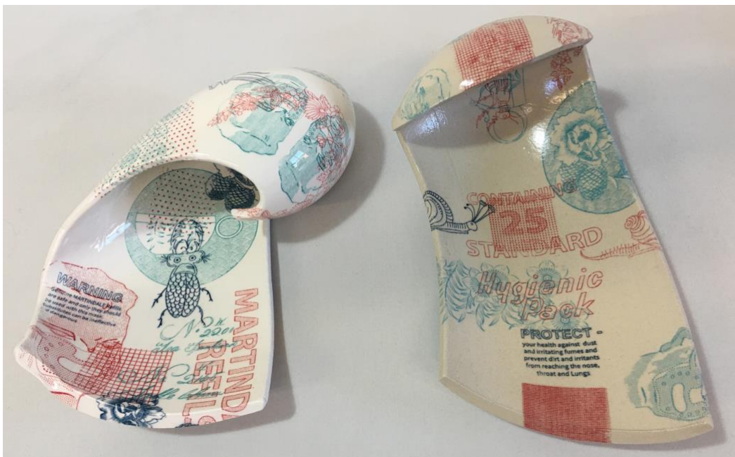
Fig.281. The differences in the clay bodies: the stoneware has fired to a dark cream toned clay body, which is a cruder and textured printing surface. The glaze surface is an eggshell finish rather than gloss one, which suggests another artistic and creative choice for tissue transferware
