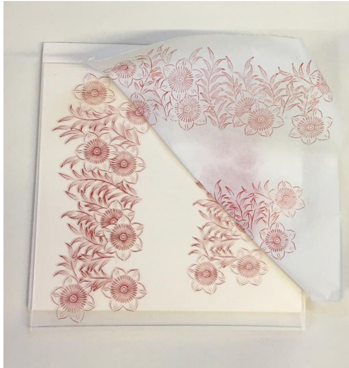
Fig.217. The printed tissue was gently peeled back from the plate to reveal the printed pattern ready for transferring
