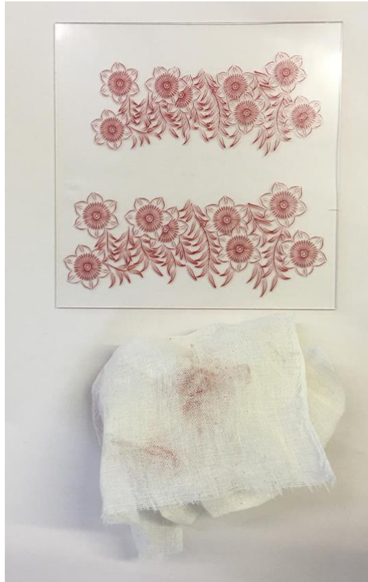
Fig.206. The final wipe from the scrim polished the plate's upper substrate to remove all traces of ink
