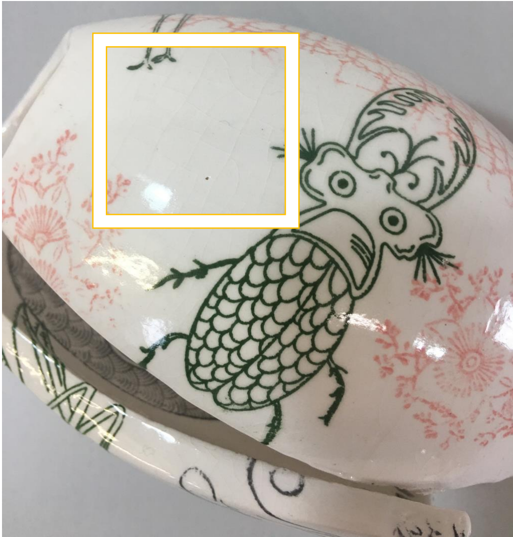
Fig.265. Firing schedule: biscuit 1000°C, hardening on 1000°C, glaze 1080°C.
