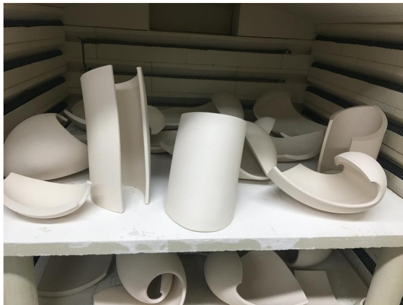
Fig.192. Two views of the ceramic shapes air dried and packed into the kiln
