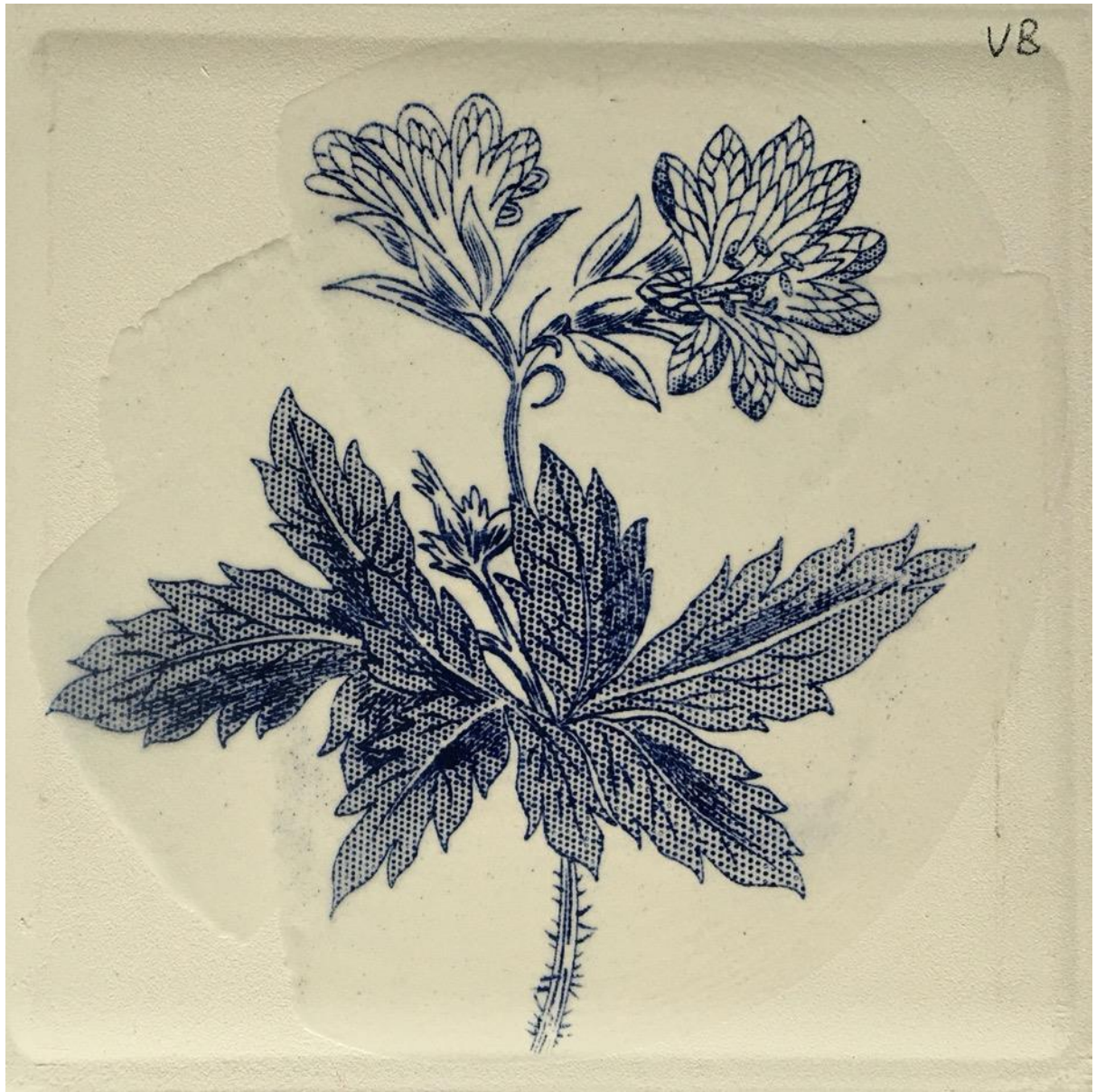
Printed design with ink: 7g Mason Stain, 3g .flux, vacuum-bodied linseed oil
