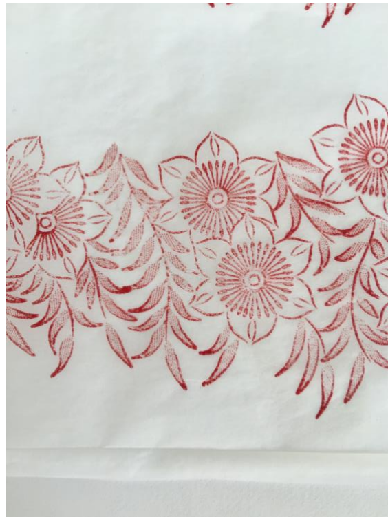
Fig.218. The tissue printed image was scrutinised and checked for uneven printing and patches of ink
