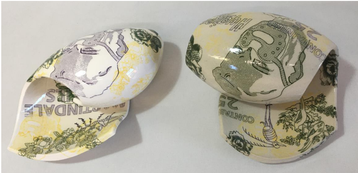
Fig.280. The differences in the clay bodies: industrially, tissue transferware utilised earthenware as a clay body as it emulated the whiteness of more expensive wares such as porcelain and bone china. The coloured prints are accentuated more on the earthenware's white background and the glaze surface is glassy and bright
