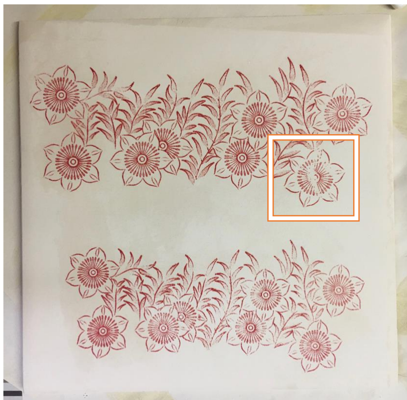
Fig.228. The print transferred effectively onto the tile with no distorting or blurring of the printed image. The fault highlighted on the printed tissue was now permanently in the printed pattern
