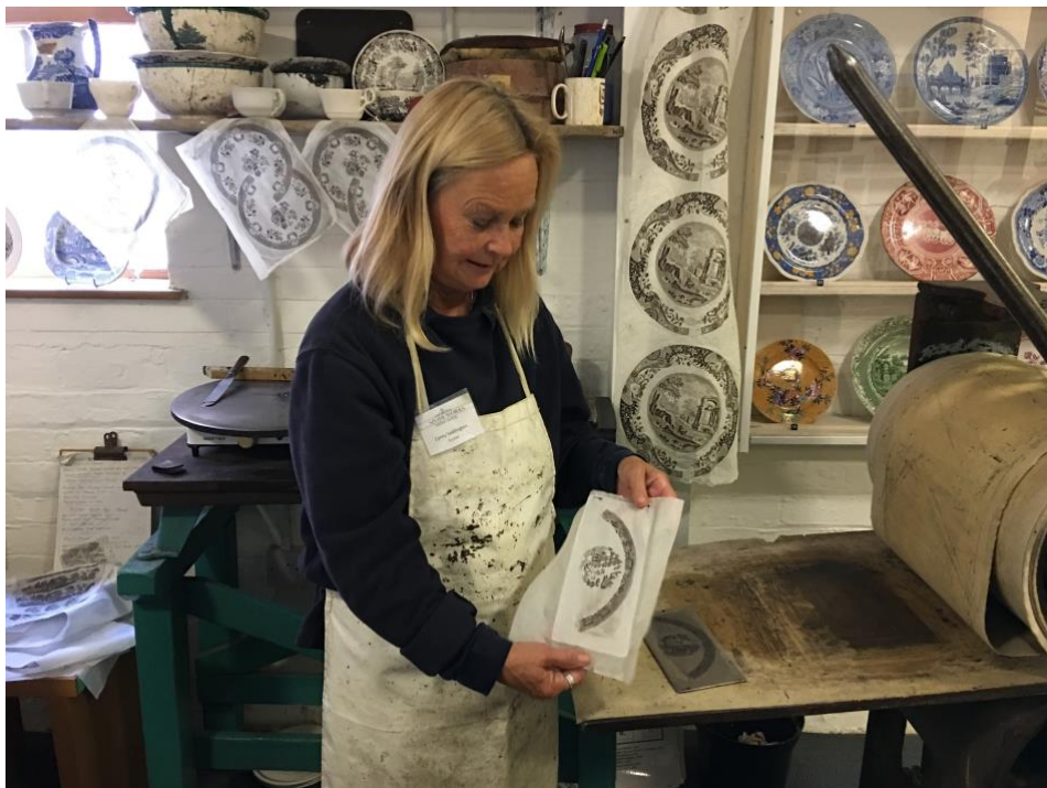
Fig. 63. The printed tissue is removed from the plate
