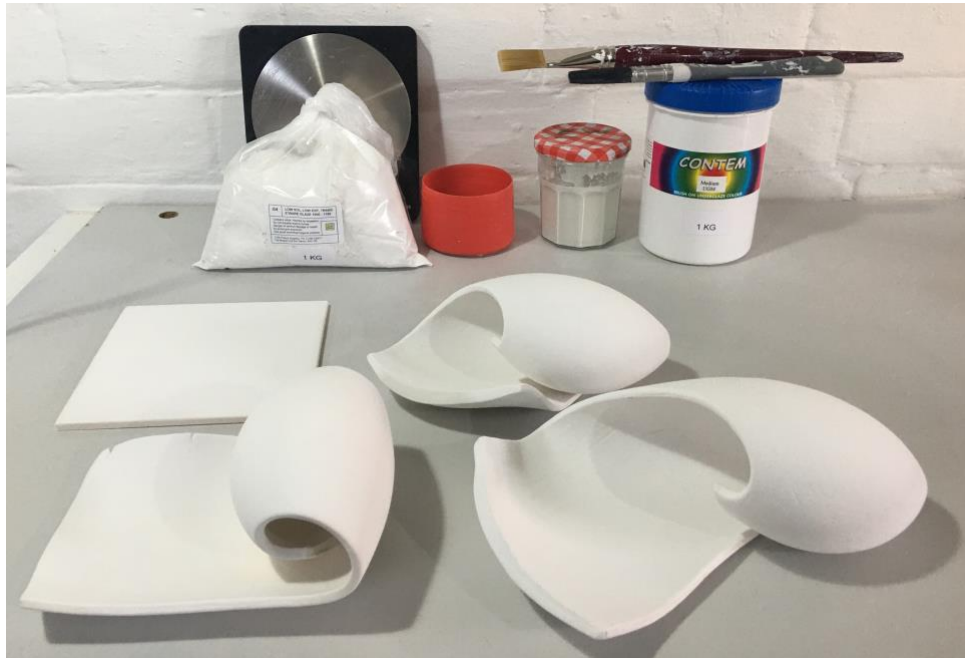
Fig.264. The transparent glaze mix was applied with a brush. The use of the medium for this mix enabled the glaze to be applied with a smooth finish. In the past when testing the process this had been difficult to achieve with a mix of dry powdered glaze and water
