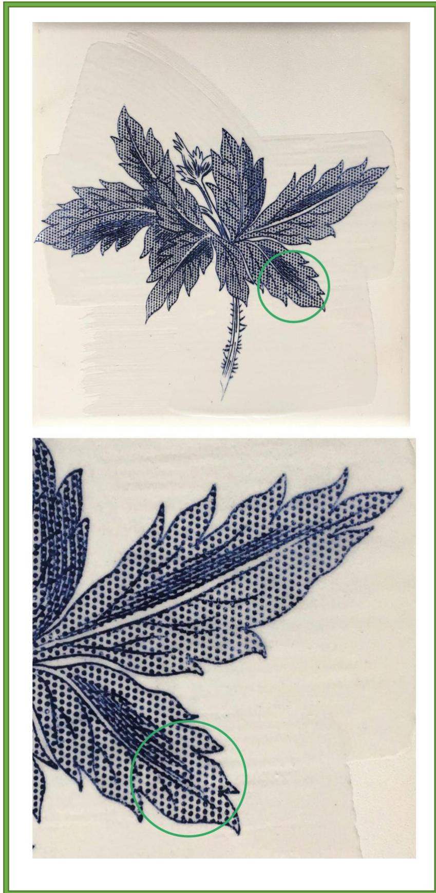
The resulting print highlighted a more open dot mark, created with a pattern swatch tool. The ink was the same formulation as Test One, changing the flux to colour ratio 3:7
