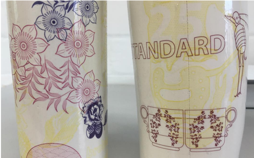
Fig.290. The printed ceramic on the left has been fired, resulting in a fused magenta printed pattern. The ceramic on the right has not been fired and shows the difference in colour from the pre-fired transfer
