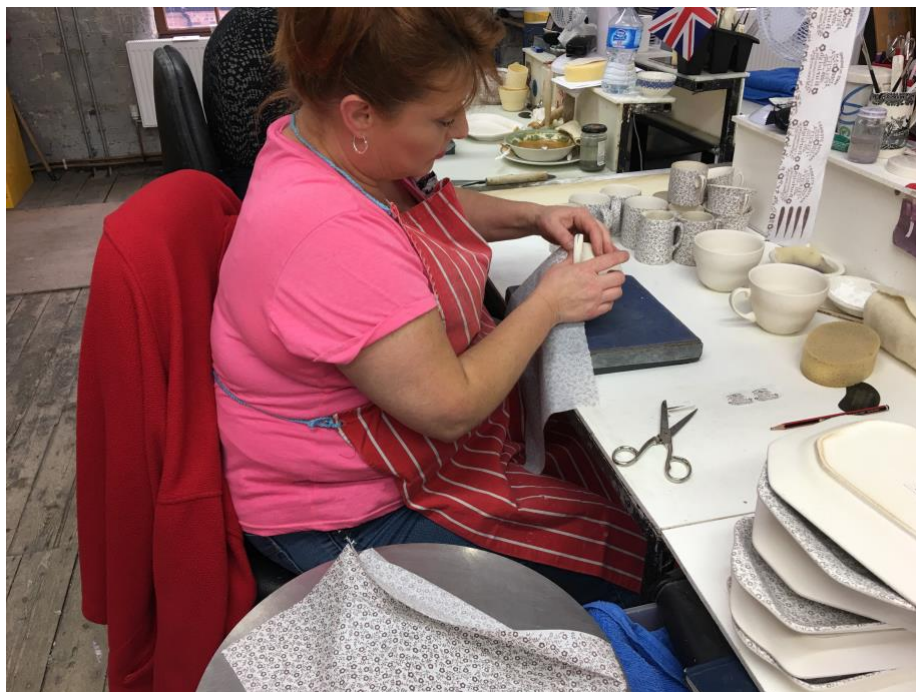
Fig. 69. The sheet of printed tissue is placed on the biscuit surface following the contours of the cup
