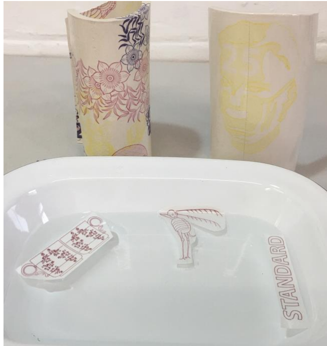
Fig.288. The transfer is released from the backing paper when immersed in water
