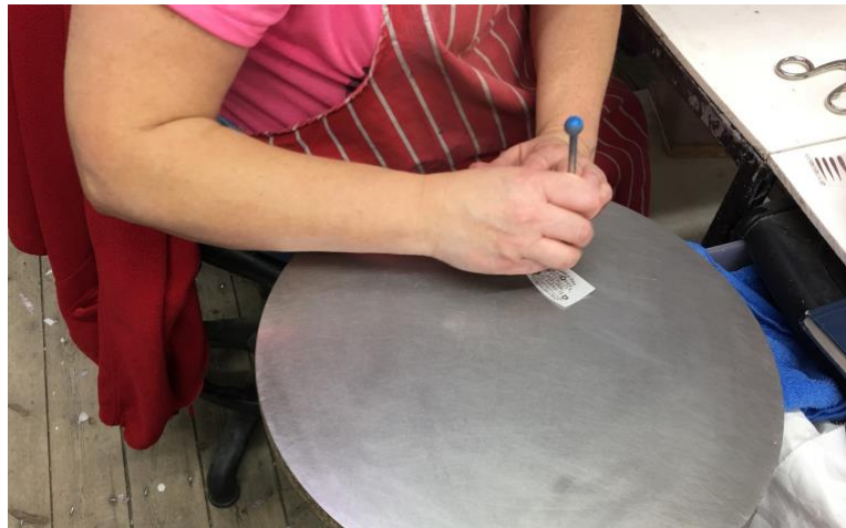
Fig. 68. The printed tissue is delivered to each transferor in lengths from the mechanical roller printer. The tissue print back stamp is cut out to be placed on the bottom of the cup
