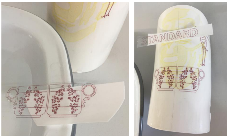
Fig.289. The transfer slides from its backing paper with a thin layer of glue remaining on the back surface to assist the image positioning. The transfers are fragile at this point and can easily tear, so care is taken when handling. The transfers are blotted with absorbent material and left to dry for 24 hours
