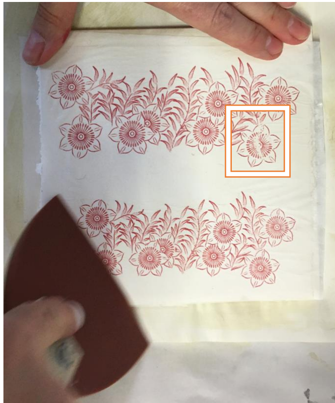
Fig.224. The highlighted area did not print effectively onto the tissue: this would be seen as a fault in the final printed ceramic
