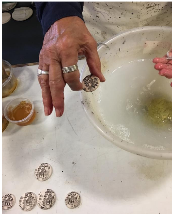
Fig. 65. When dry the printed disc is submerged in water the tissue dissolved into the water revealing the print on the ceramic
