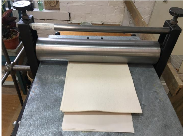
Fig.215. A stack of four etching blankets: placed on top and secured in the roller
