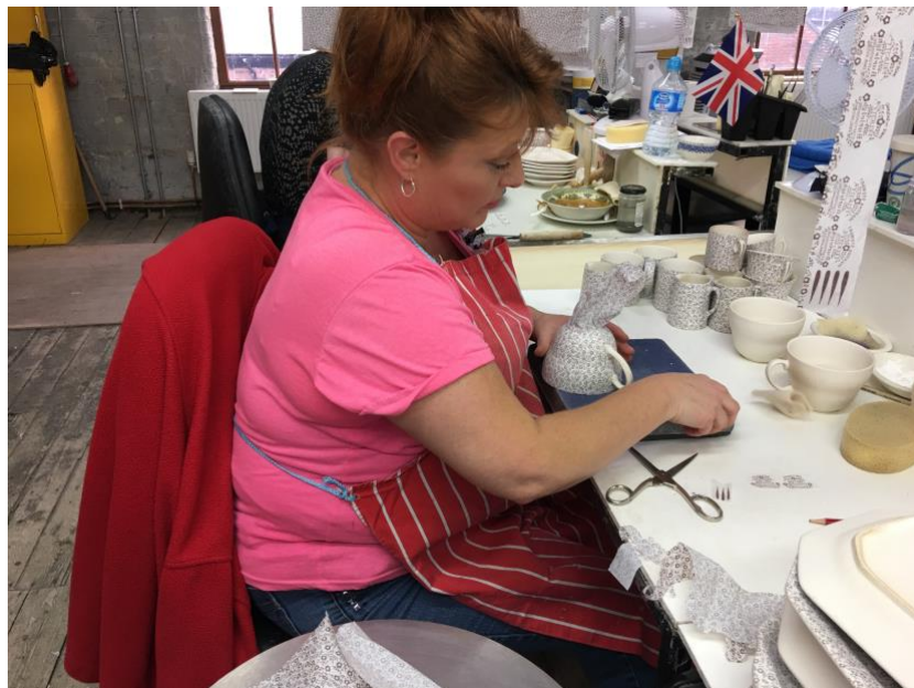
Fig.71. The whole surface is covered with the printed tissue and rubbed down with a stiff brush
