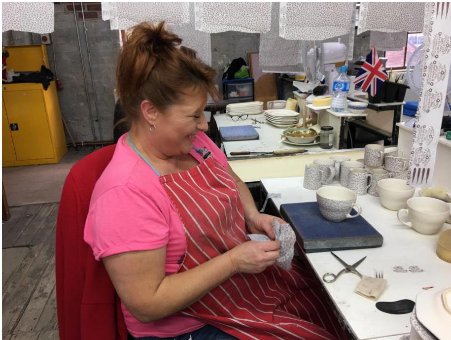
Fig.73. The cup is now ready to be dried and tissue washed off to reveal the printed pattern
