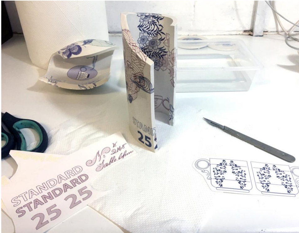
Fig.292. The image is accumulative, with the transfers sitting on the uppermost gloss glazed ceramic surface
