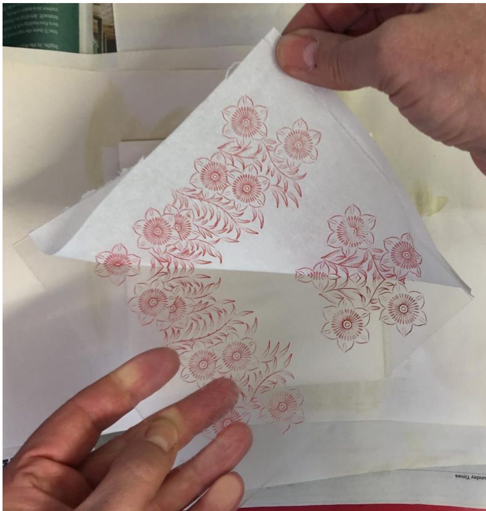
Fig.219. When the tissue was released from the plate it was flimsy and likely to stick onto itself, so it needed to be handled quickly and efficiently and placed into the final printing position
