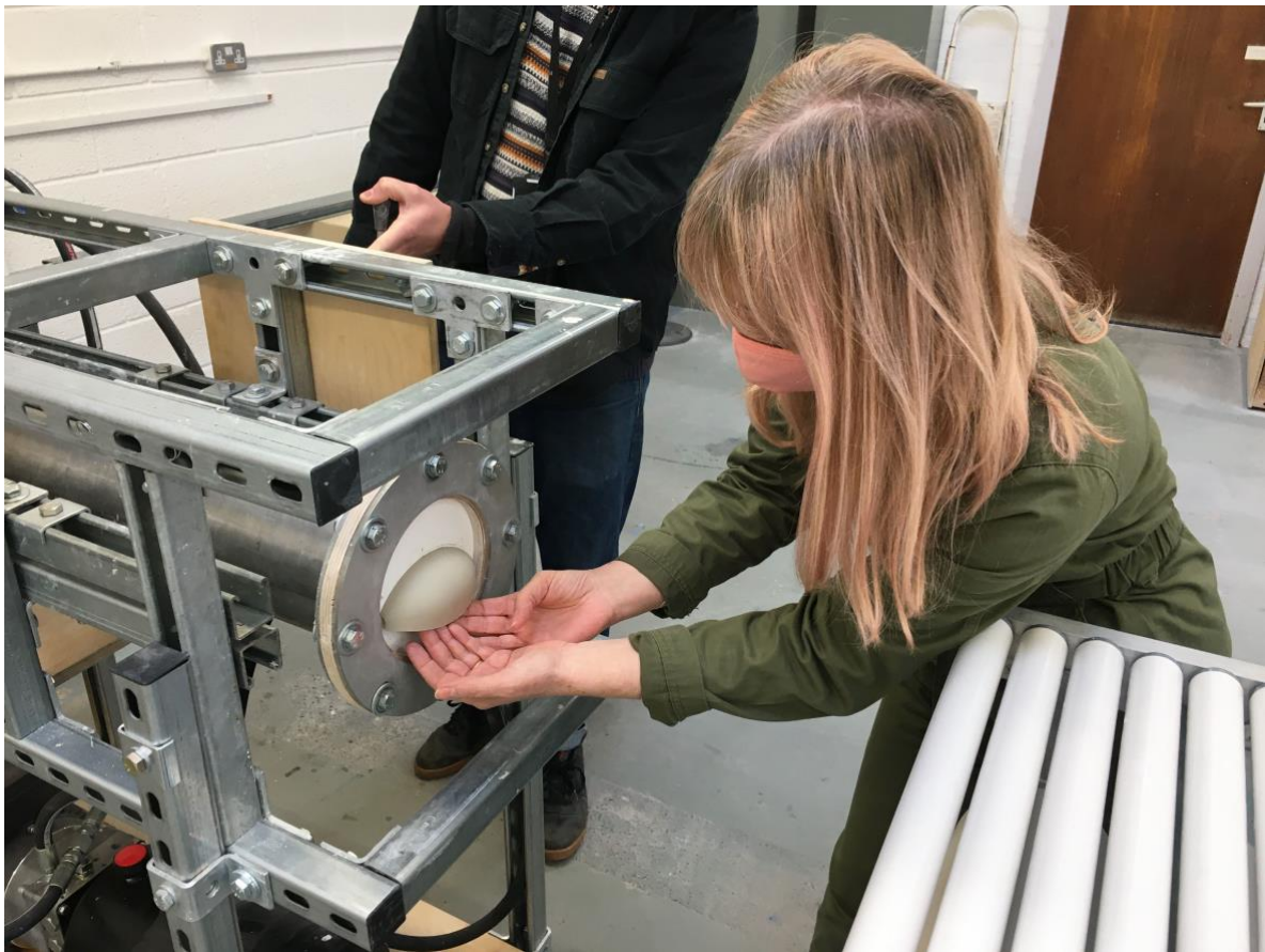
Fig.188. The clay moved slowly through the extruder with the hydraulic pump powering it through the die to form a shape
