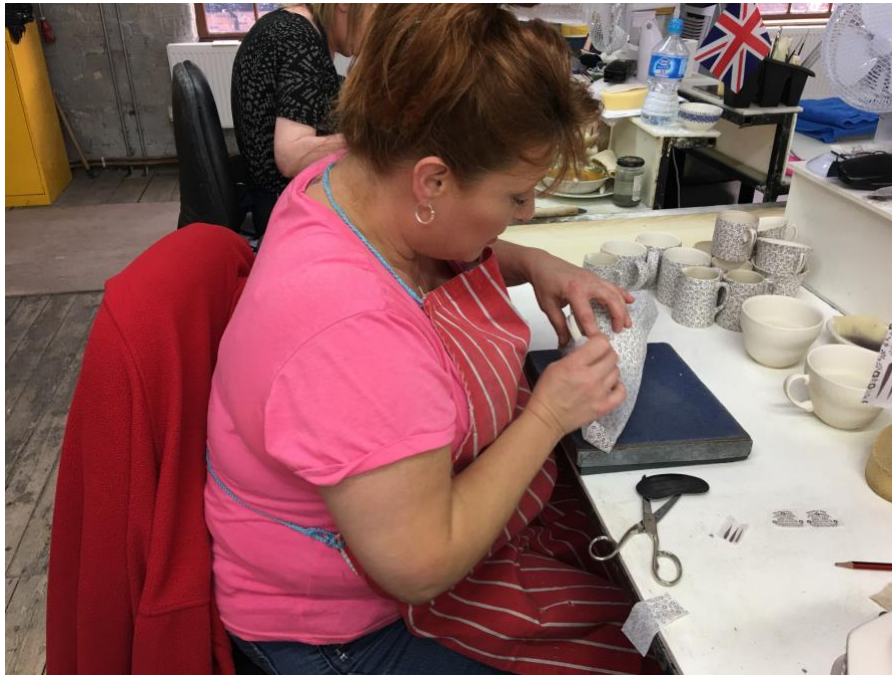
Fig. 70. The transferor wraps the print around the compound shape of the cup and secures it with pressure from a silicone kidney and damp felt pad
