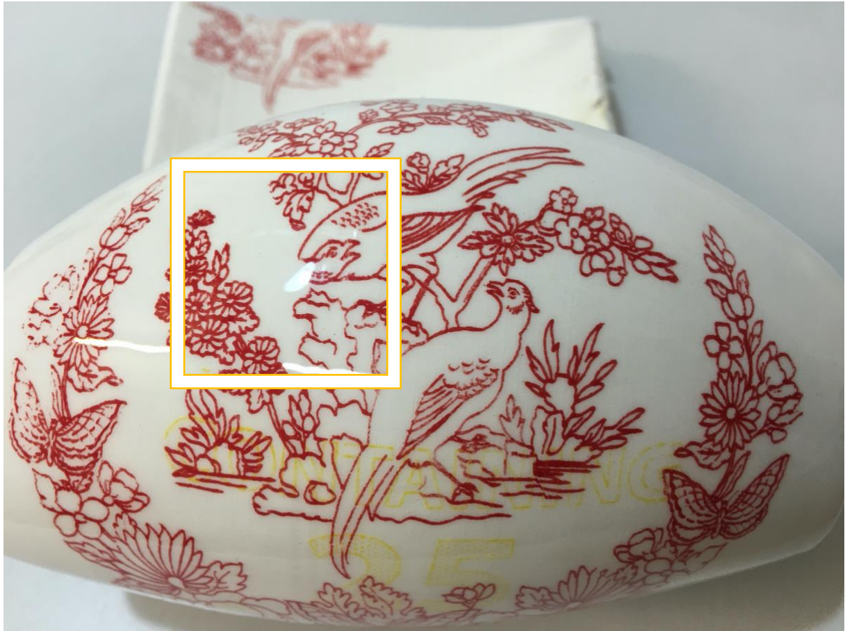
Fig.266. Trialling this industrial method: the crazing on the glaze ceased by hardening on the print at 1120°C and glazing at 1080°C
