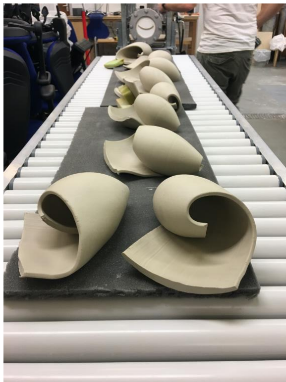
Fig.190. Two views displaying supporting the clay shapes with sponge formers until the clay was leather-hard and could be modelled further
