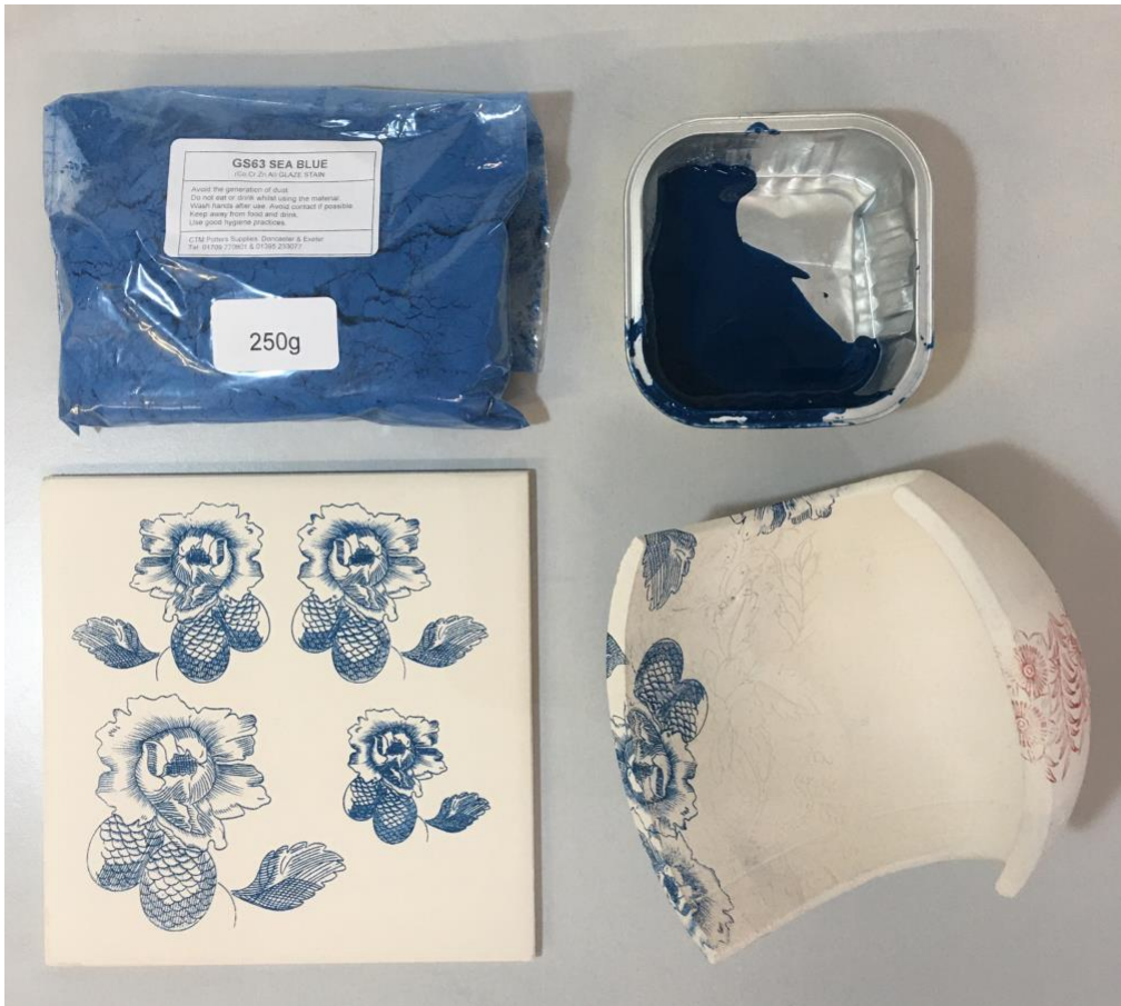
Fig.238. The ink was mixed using CTM GS 63 Sea Blue
