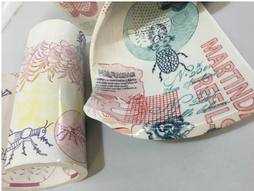
Fig.301. The differences between both types of transfer printing, with the on-glazed piece to the left
