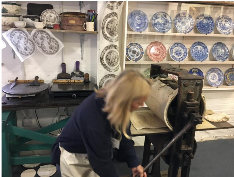
Fig. 62. The plate and tissue are covered with the blankets and pulled backwards and forwards through the engraving press
