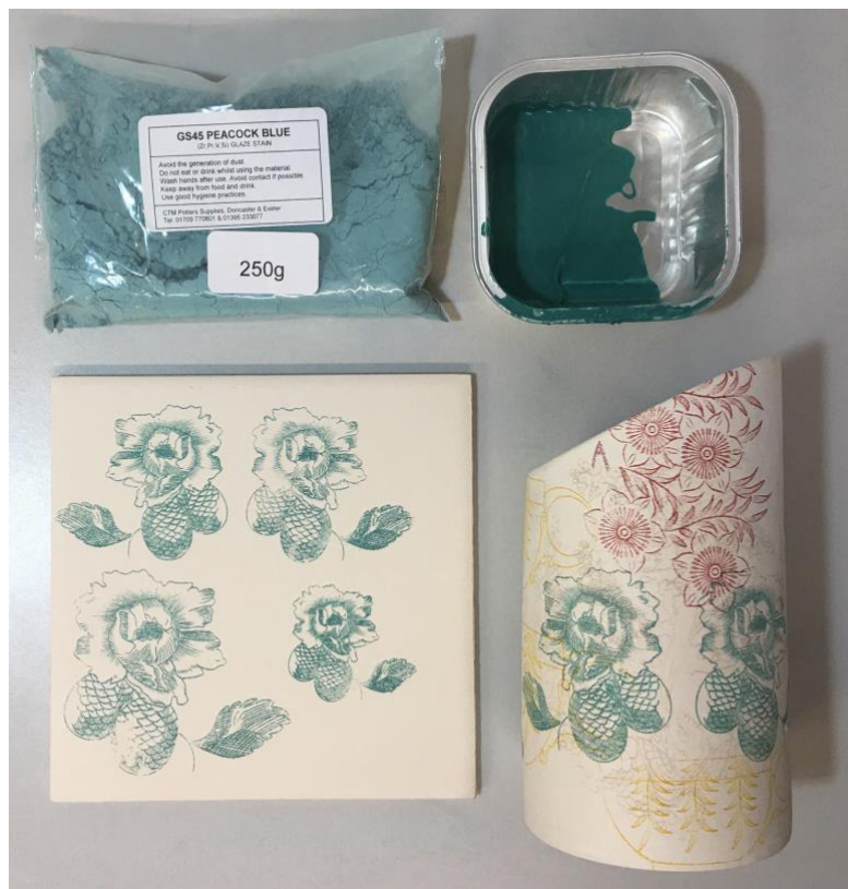
Fig.233. The ink was mixed using CTM GS 45 Peacock Blue
