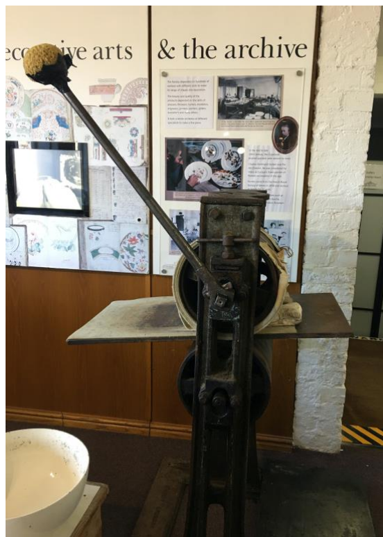
Fig. 57. The original press used for demonstrations by the Spode Trust. The printing uses an intaglio method, and the printing press is very similar to one used for etching and engraving on paper (reproduced by kind permission of The Spode Trust), photographed by Lisa Sheppy, Stoke-on-Trent,
