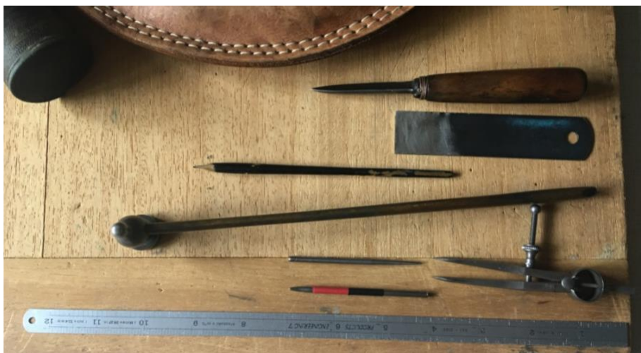
Fig. 33. Paul Holdway's engraving tools: used for many years at Spode and still used by him today. In this photograph, from the bottom of the image is a ruler, burin or graver, compass, hammer, pencil, small ruler, and scraper.
