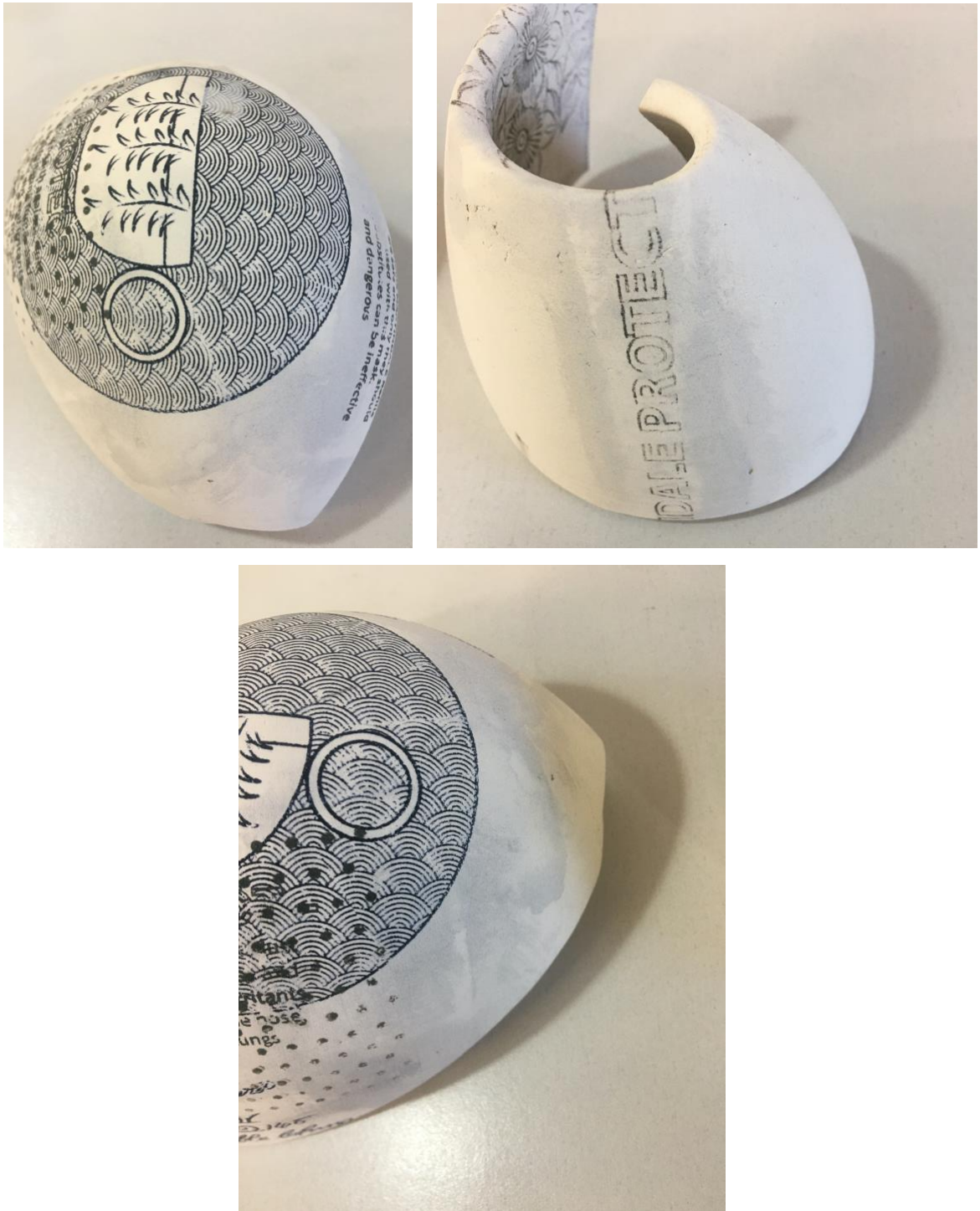
Fig.249. Three views: the results of the 3D earthenware shapes biscuit fired to 1150°C indicate that this temperature was too high for the transfer printing to be effective. The biscuit fired form was unreceptive to the transfer print and repelled the print from the ceramic surface. The further hardening on firing of 1000°C resulted in an inconsistent and discoloured print on the ceramic
