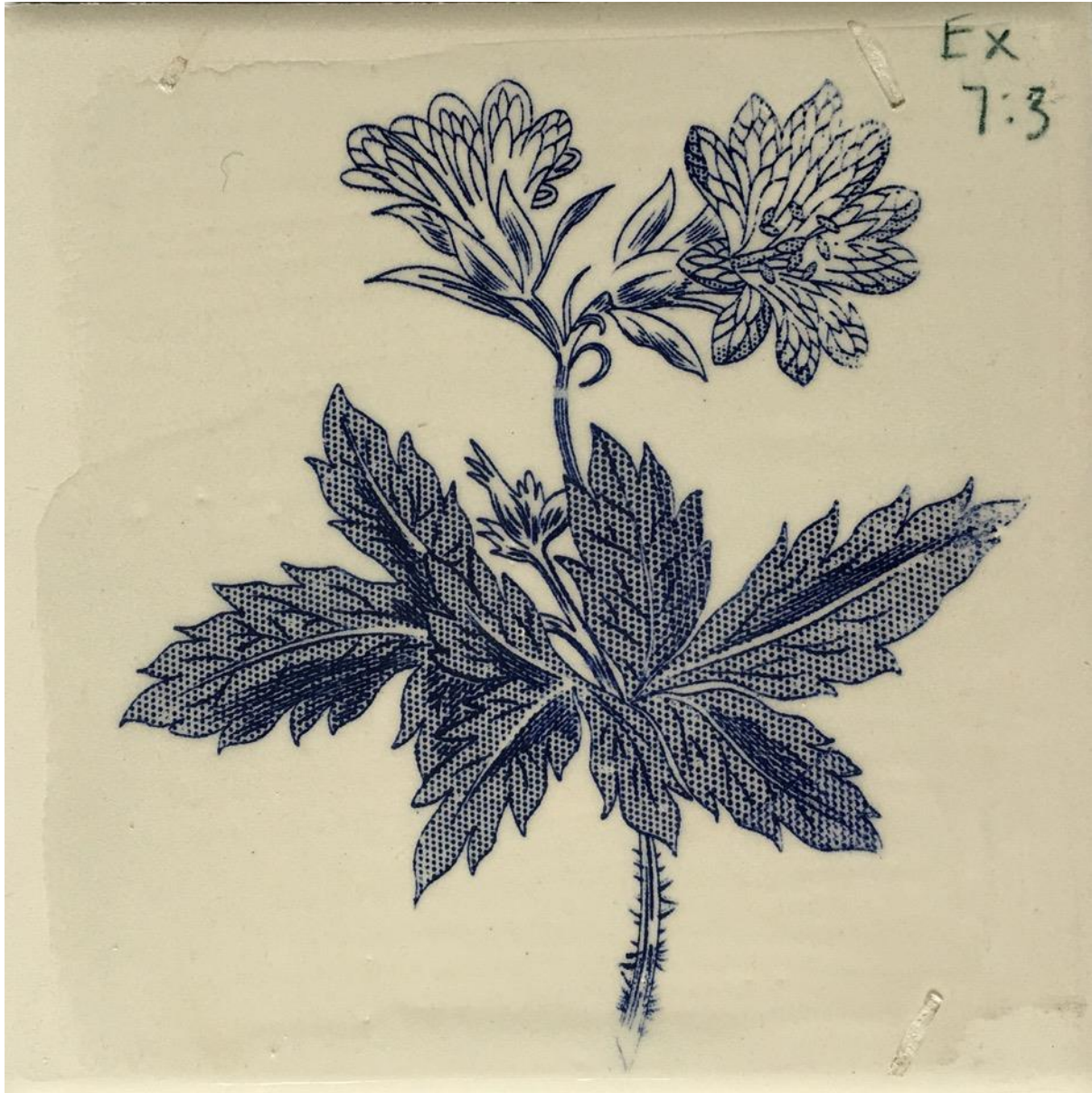
Printed design with ink: 7g Mason Stain, 3g flux, extender
