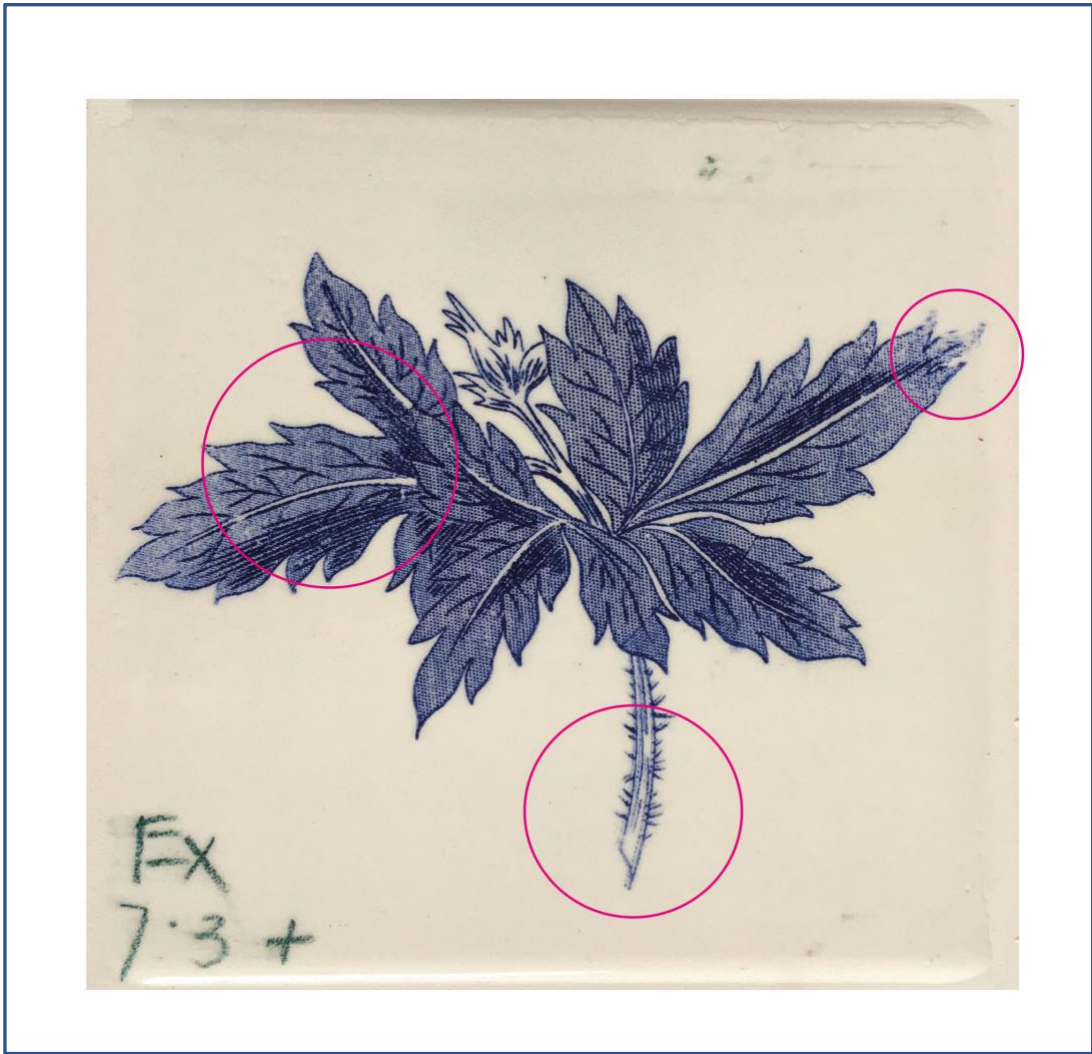
The outcome of Test Two: inked, printed, transferred, hardened on fired and glaze fired, highlighting issues with the printed image
