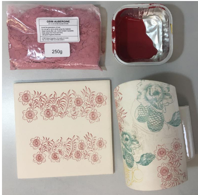
Fig.232. The ink was mixed using CTM GS 56 Aubergine
