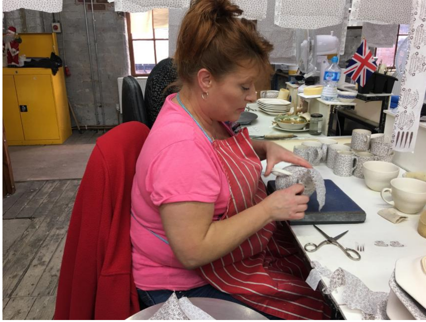
Fig.72. The excess tissue is cut away from the cup, forming a neat edge
