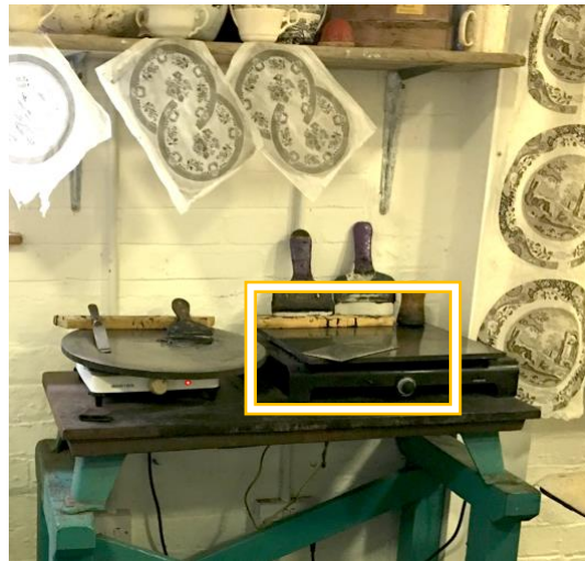
Fig. 60. Hot plates in the Spode Museum Trust Heritage Centre are used to heat the plate and ink. The plate is inked up intaglio with a ready mixed product which contains the cobalt oxide colourant and an oil carrier. This is a hot process which is carried out on warm plates to assist the inking process
