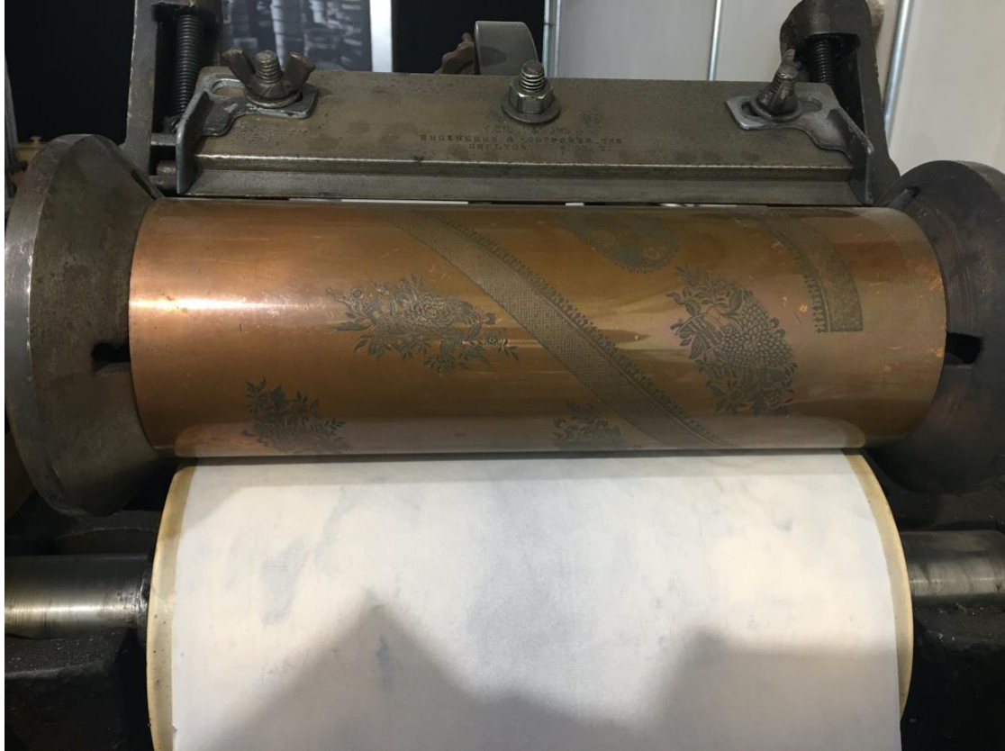
Fig.78. Redundant Pottery Printing Machine . The ink is applied manually into the well at the top of the engraved roller using a palette knife. The scraper blade below the well removes the excess ink before the tissue passes through the inked rollers. Photographed by Lisa Sheppy, Spode Museum Trust Heritage Centre, 2019
