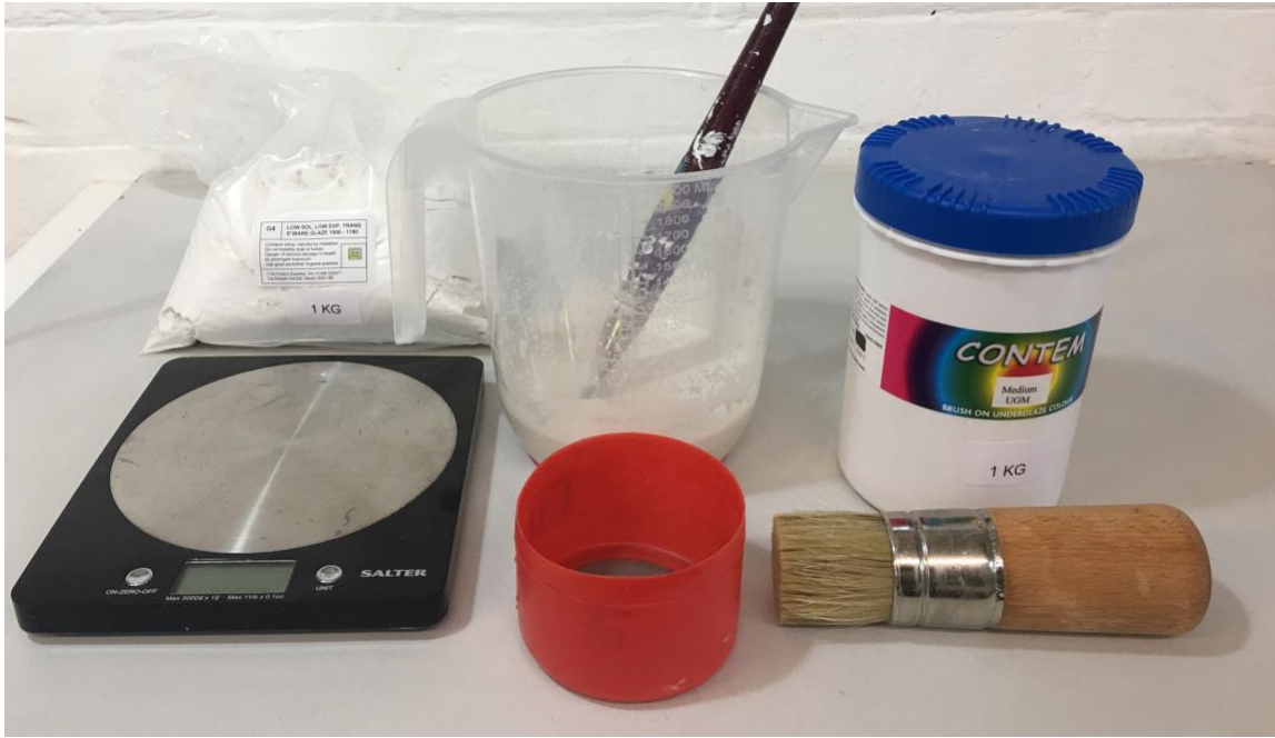
Fig.256. The glaze powder was mixed with water and a universal medium which acted as a flocculant , resulting in a smooth glaze which could be applied with a brush. The ratios for this were: 50gm powdered glaze, 40gm water and 40gm medium, and the glaze mix was passed through a fine sieve to become ready for application
