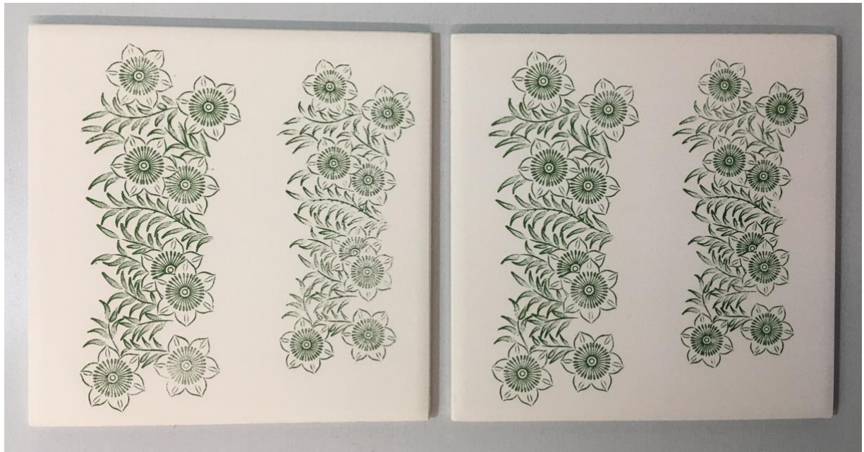
Fig.248. CTM GS 3 Green ink: shows how the print can differ slightly during the process of printing and transferring
