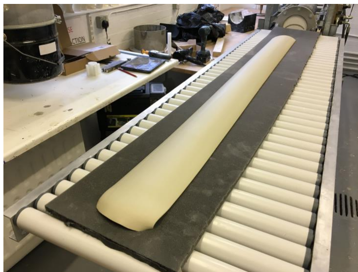
Fig.187. Two views of the of the extruded continuous clay form produced through the steep and shallow die profiles
