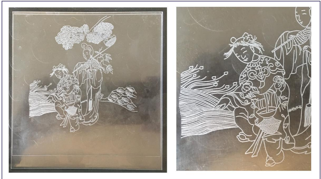
Fig. 122. Laser engraved plate used for tests. The Illustrator file was emailed and exported to Laser Lab, Bristol . The design was laser engraved onto a 2mm acrylic sheet and sent by post back to me
