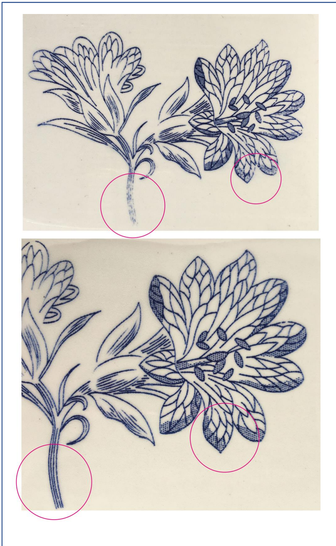
The outcome of Test Two: inked, printed, transferred, hardened on fired and glaze fired, highlighting issues with the printed image
