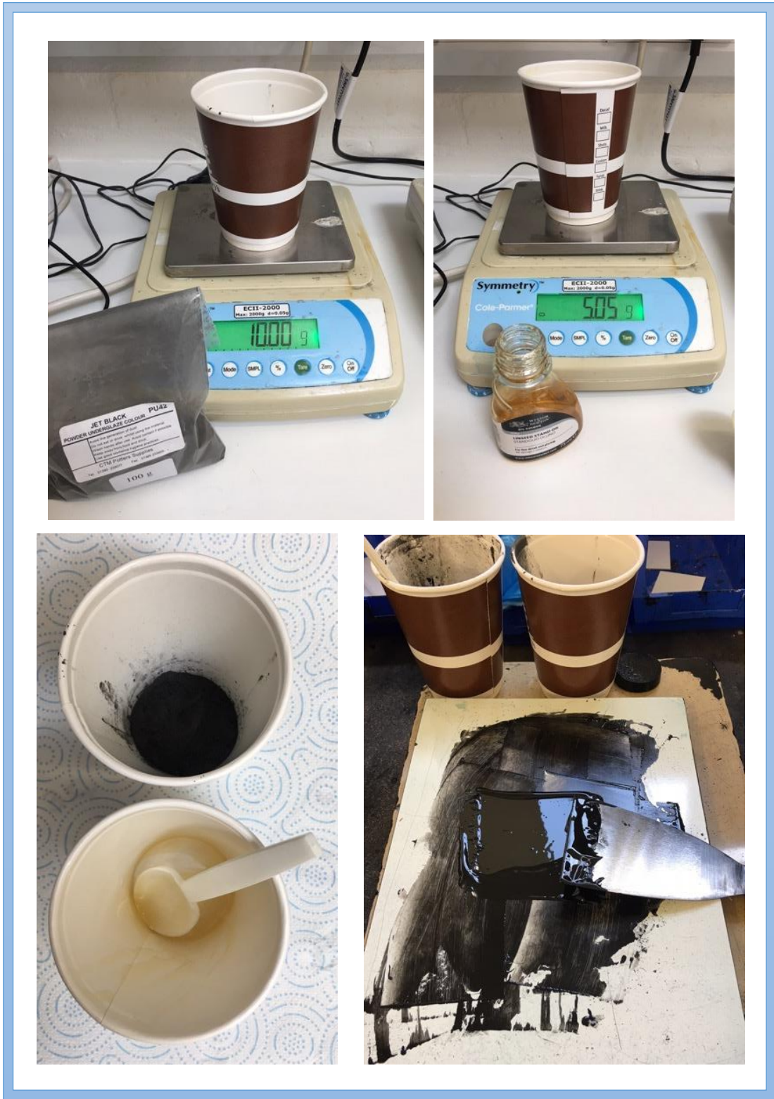
Mixing ink based on a recipe suggested by Petrie (2011: 110), 5g oil to 10g stain plus lineeed stand oil
