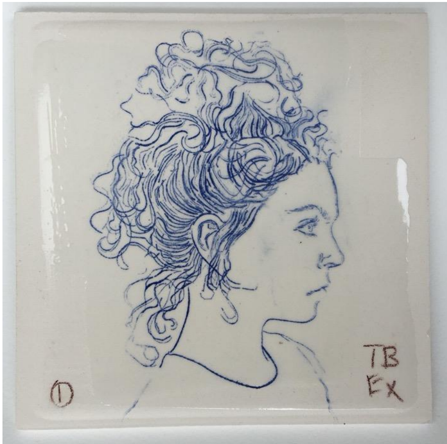
Resulting ceramic test highlighting issues with the transfer, as the print has blurred.
