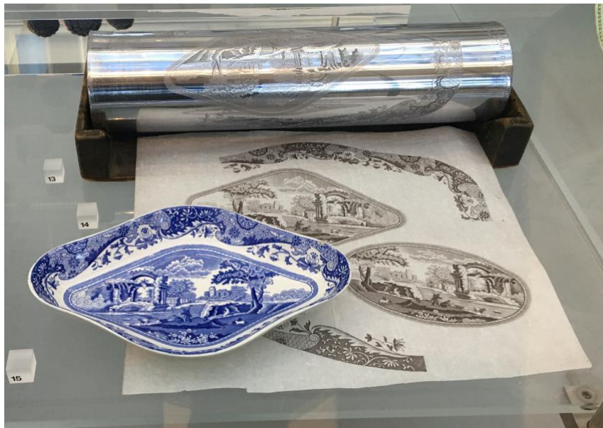
Fig.75. Engraved copper roller with Blue Italian pattern, Staffordshire, 1975. Roller engraved at Spode's factory by Paul Holdway, chromium-plated with wooden stand, photographed by Lisa Sheppy 2017. ©Victoria and Albert Museum, London
