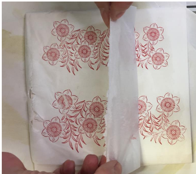
Fig.227. The tissue was released from the ceramic tile, revealing the print on the ceramic tile
