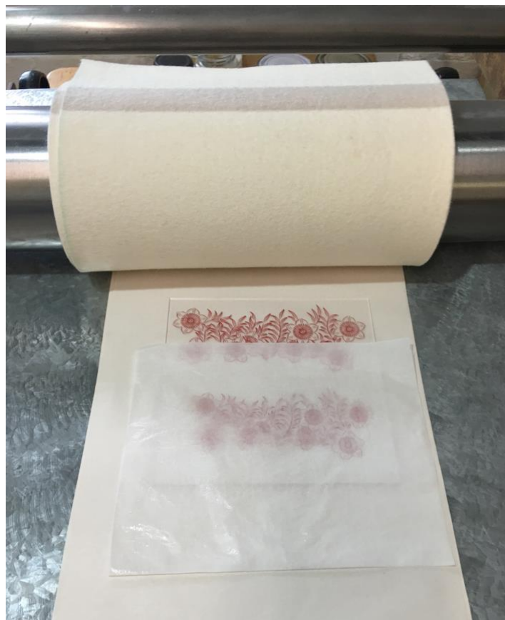
Fig.212. The tissue was placed on top of the inked-up plate with the soap layer up
