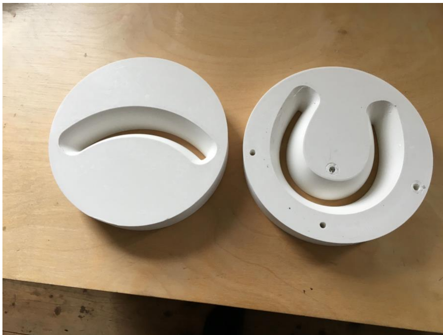
Fig. 186. The two dies were 3D printed into steep and shallow curves based on my discussions with Jorgensen and Lightfoot
