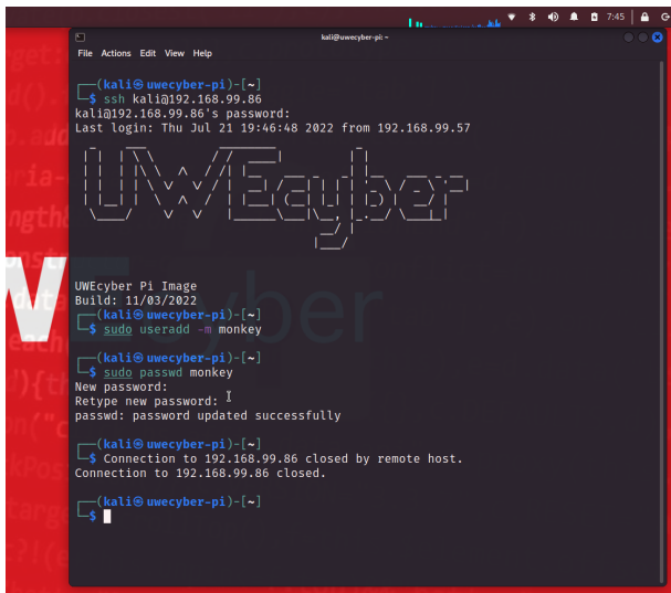
Fig. 9. Red team remotely access the target and create a new user account before being disconnected by the blue team.
