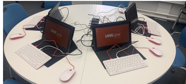
Fig. 1. UWEcyber Pi Lab portable setup, consisting of 4 Raspberry Pi 400 devices with portable monitors and a Raspberry Pi 4 access point.
