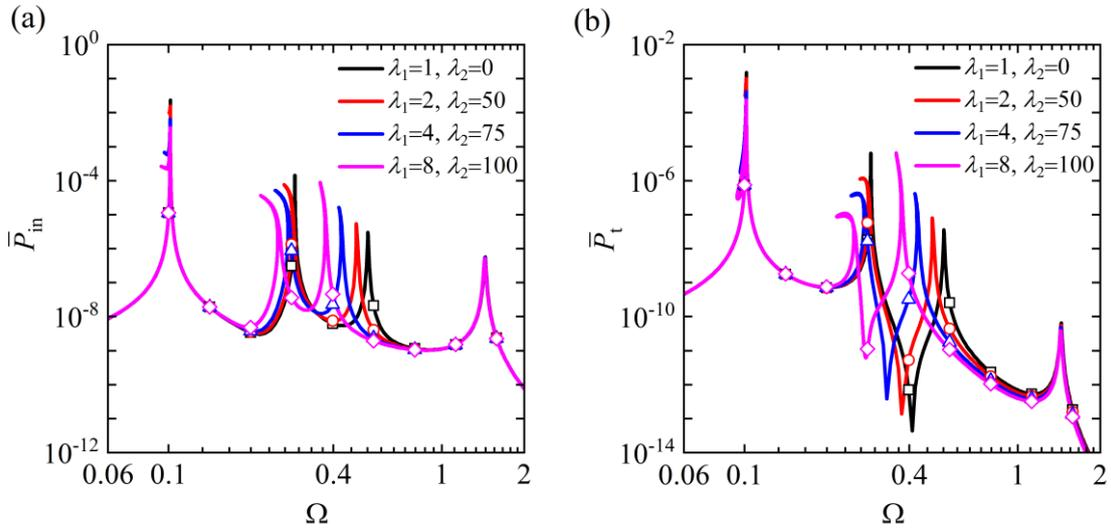
315 **Figure 7.** Effect of TMDI with different inertance combinations on the (a) input power  $\bar{P}_{in}$  and (b) power
