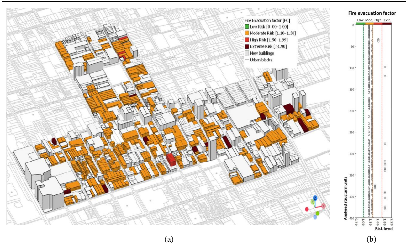
566 Figure 10: (a) Mapping and (b) results of fire evacuation analysis of Yungay typical zone
