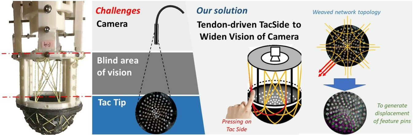
Fig. 2. MechTac. For solving the perceiving tactile information out of field of view (blind area of vision), we use tendons to weave on a net connect the TacTip and the pressing regions. when you press on different regions on the skin the associated tendons are tightened to modify the distributions of the pins on the TacTip to generate displacement of feature pins.
