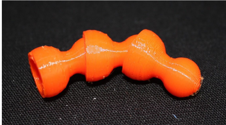
[Figure 30. FDM printed joint in NinjaFlex flexible filament.]
