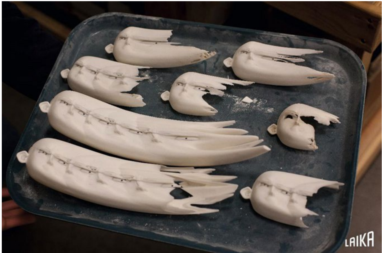
[Figure 12. Individual smear frames printed to create dynamic in-camera special effect for ParaNorman (2012). Image used with Special Thanks to LAIKA Studios]
