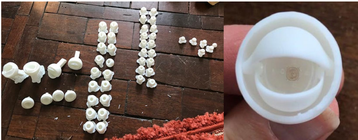
[Figure 56.1. Left: Printed piece for all sets. Figure 56.2. Right: Constructed 10.4mm eye with white and elastic resin. Images used with thanks to Ainslie Henderson.]
