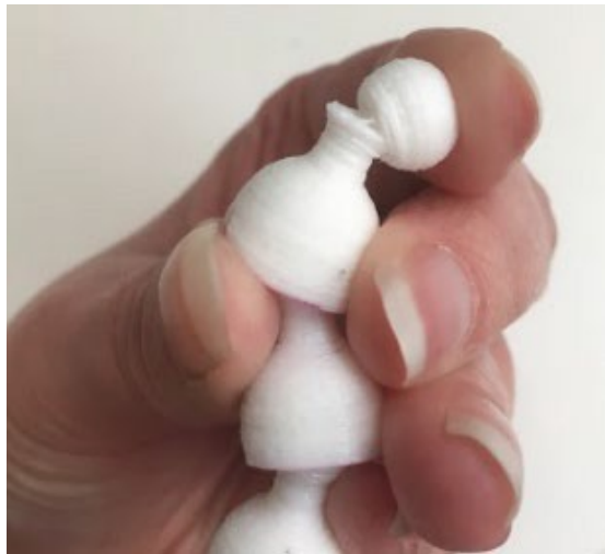
[Figure 29. Tear in neck of FDM flexible print]
