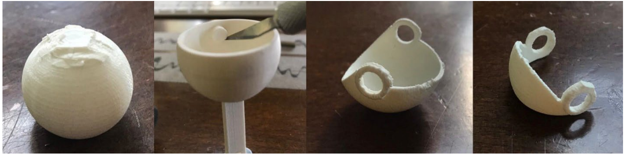
[Figure 43. 3D Printed test of second design, FDM printed in PLA. Images used with thanks to Ainslie Henderson.]
