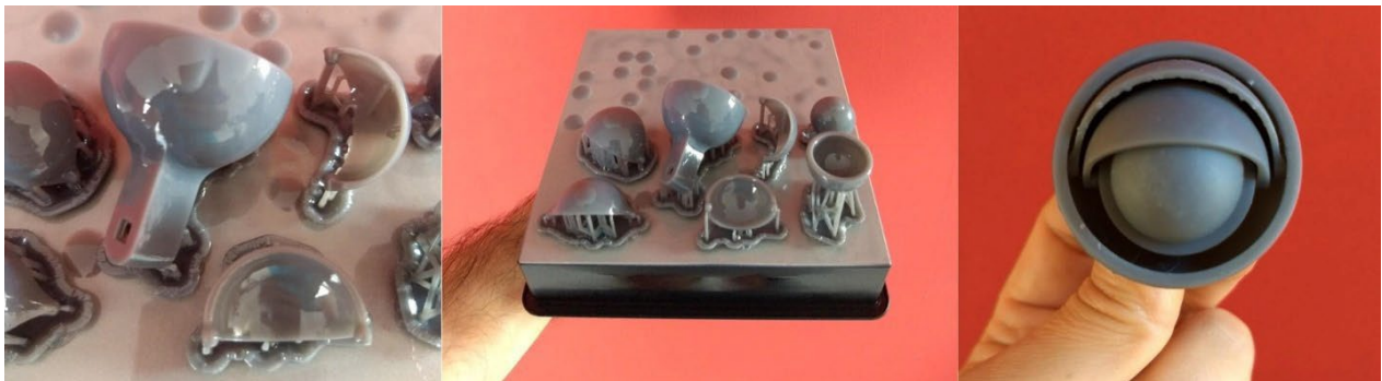
[Figure 47. Test prints of 20mm eye system in grey resin Formlab 3. Images used with thanks to Fabio D'Agnano.]
