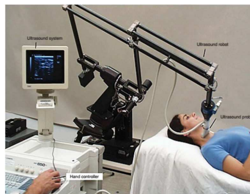
Fig. 5 Robotic arm for teleoperated ultrasound [8, 10]
