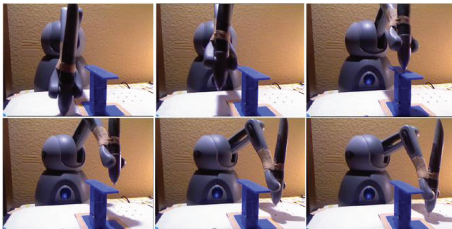
(c) Robot crosses 3-block height obstacle avoidance autonomously
