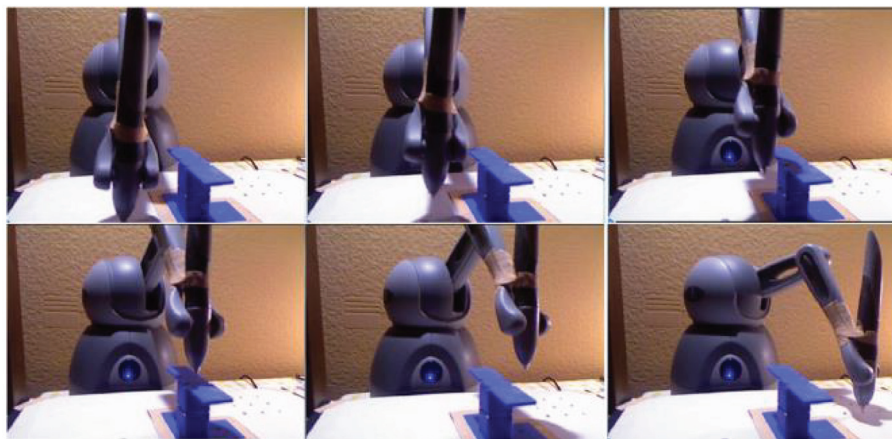
(b) Robot crosses 2-block height obstacle avoidance autonomously
