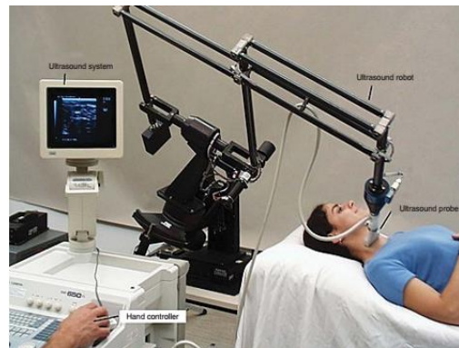
Fig. 5. Robotic arm for teleoperated ultrasound([18],[20])
