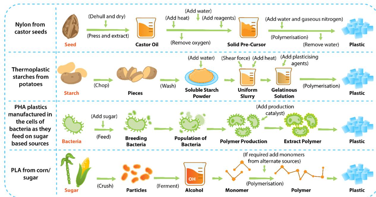
Figure 3. Different production routes for bio-based and biodegradable polymers.<sup>81,82</sup>
