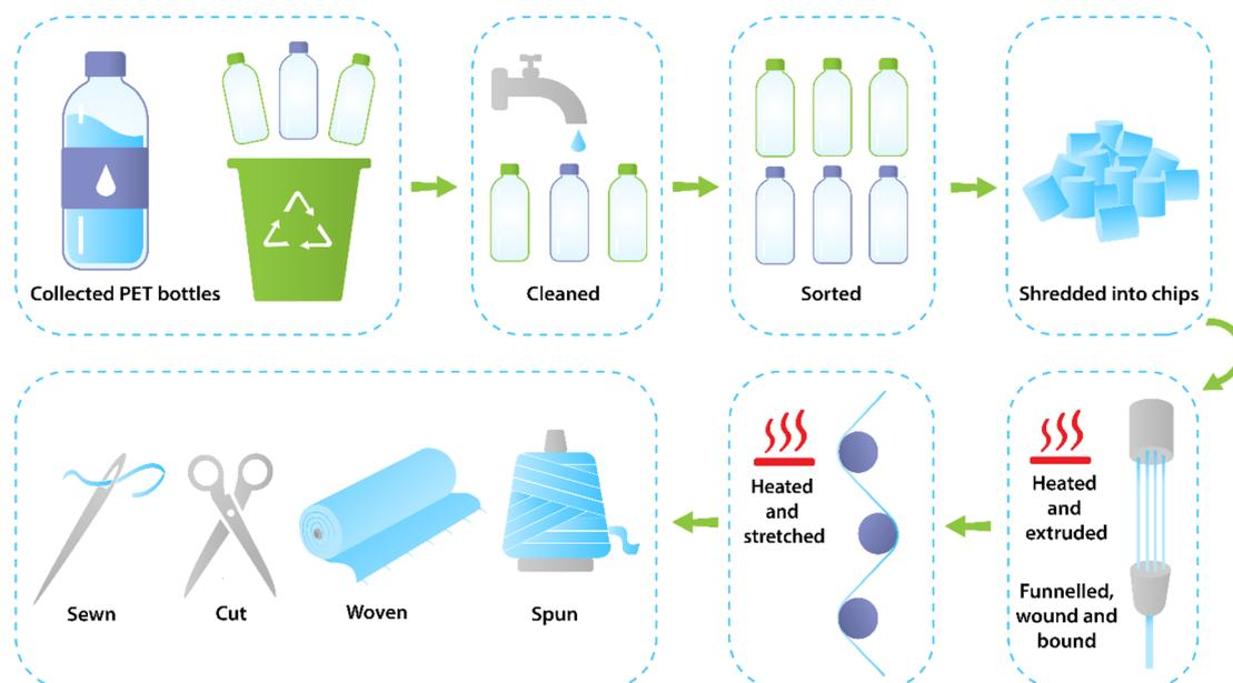
Figure 2. Process flow: from collection of PET bottles to recycling into garments.<sup>64–67</sup>
