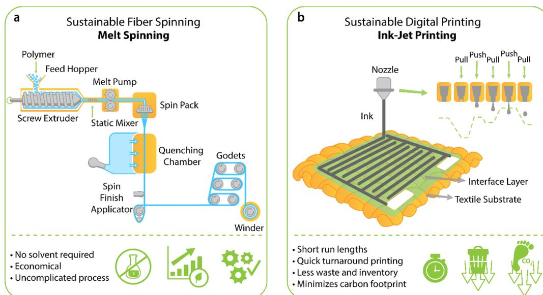
Figure 7. Sustainable manufacturing techniques: (a) fiber-spinning: melt-spinning.<sup>284</sup> (b) Digital printing: inkjet printing.
