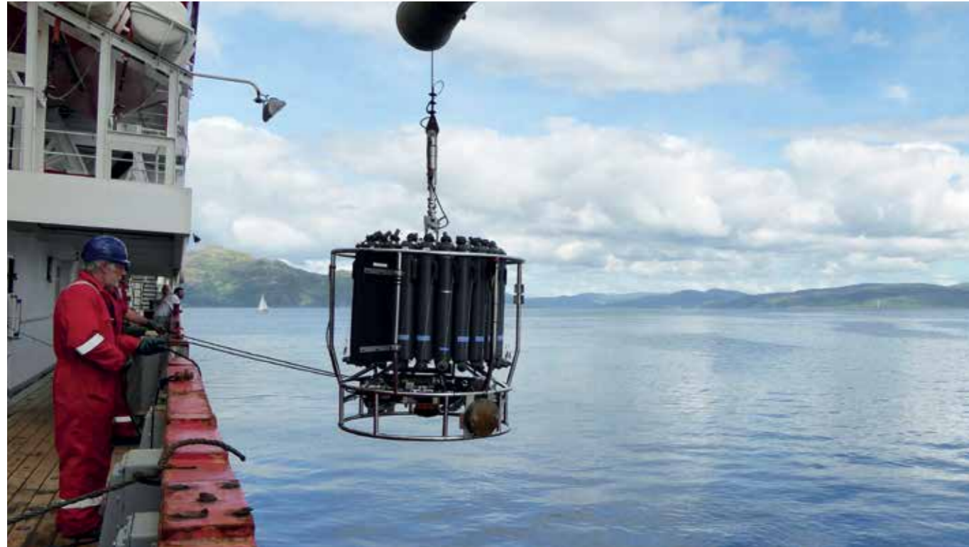
▲ CLASS scientists use a package lowered to the seafloor from research ships to measure currents, temperature, salinity, pressure, oxygen and fluorescence. The device also captures samples of water for chemical and biological analysis. (© National Oceanography Centre)
