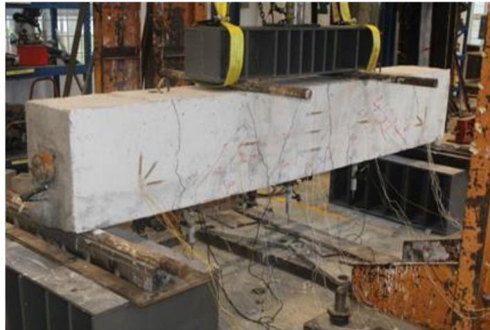
Fig. 8. Test setup of beam specimens under four-point bending test
