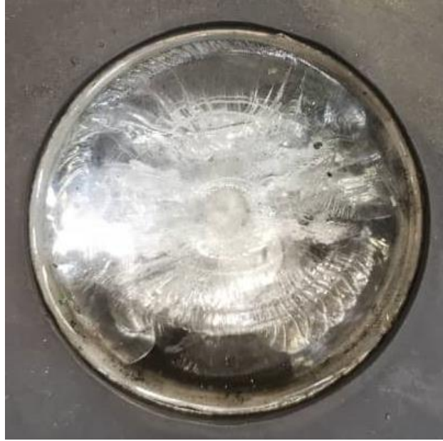
Fig. 14 Damage observed on the top of epoxy filler
