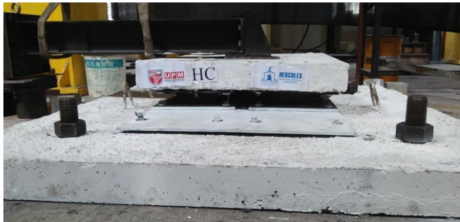
Fig. 28 Experimental testing of specimen HC under horizontal cyclic loading
