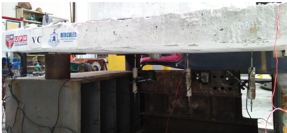
Fig. 34 The three dial gauges set under the lower slab
