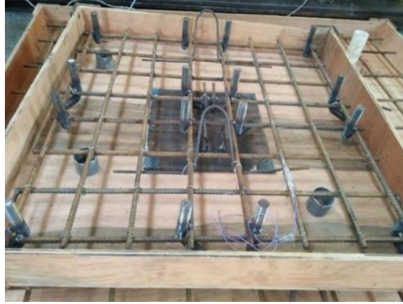
Fig. 25 Steel bolts and load plate embedded inside upper slab for horizontal test before casting
