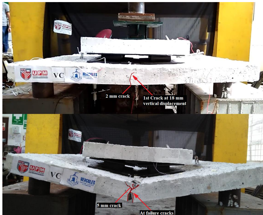
Fig. 33 Experimental testing of specimen VC under vertical half-cyclic loading
