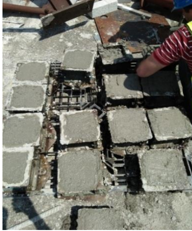
Fig. 26 Cubic concrete samples for compressive strength test
