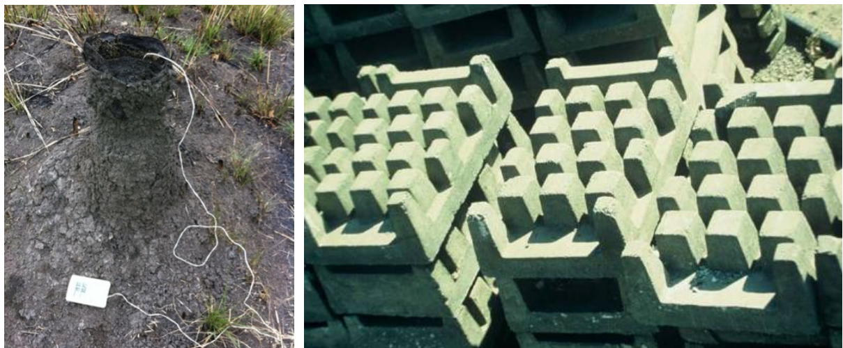
360 361 Figure 7. Temperature measurements of termite mounds carried out by Mick Pearce (left), CC0 Licence, Mick 362 Pearce. (b) Heat exchange floor under construction, abstraction of the biological principles of termite mounds, 363 CC0 Licence, Mick Pearce.
