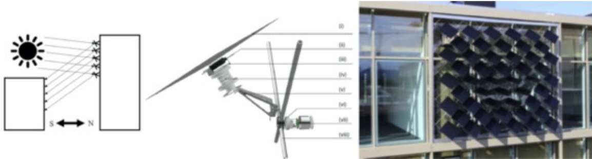
Figure 15.14. Adaptive Solar Façade (ASF). (Left) envisioned interactions between direct sunlight and buildings; (Middle) detail of the AFS panel: (i) PV panel, (ii) junction box, (iii) panel adaptor, (iv) soft pneumatic actuator, (v) cantilever, (vi) electronic and pneumatic plug, (vii) electronic shield, (viii) rod net structure incl. pneumatic tubes and wiring; (Right) The prototype ASF constructed on the House of Natural Resources at ETH Zurich. Figures reproduced from [111], with permission from Elsevier.
