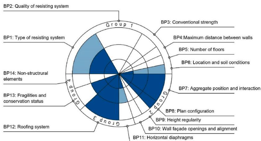
Fig. 12. Example of a graphical representation for the building SECII-27.
