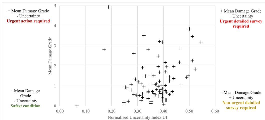
Fig. 11. Distribution of the sample according to the calculated mean damage grade against the uncertainty index.
