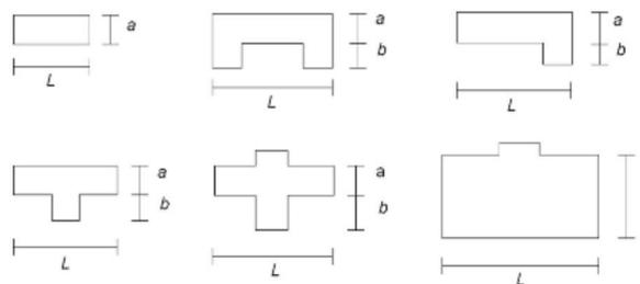
Fig. 1. Examples of L, a and b for multiple plan configurations..
