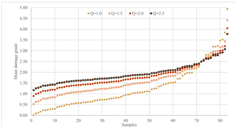
Fig. 10. Variability of the Mean damage grades for the 83 constructions by using different values of ductility Q (The buildings were arranged from the lowest up to the highest mean damage grade value).
