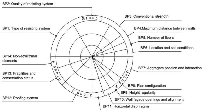
Fig. 2. Schematic representation of the parameters and their weight.
