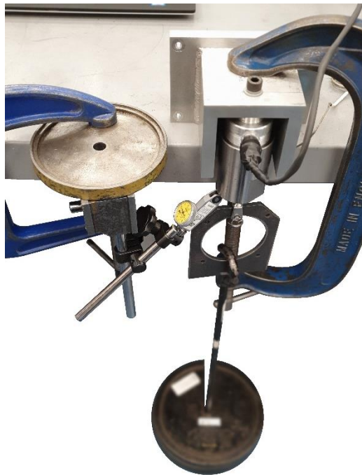
Figure 6.26: Setup for measuring voltage output V_l from load cell at different loads.
