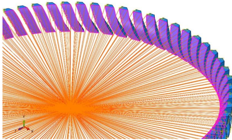
Figure 7.5: Inside faces of wheel teeth constrained to centre point of wheel gear.
