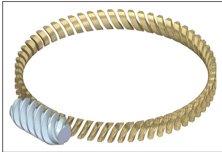
Figure 7.2: CAD model of worm gearset 3 simplified for import into Abaqus®.
