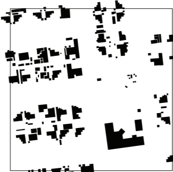
Larger villa type Al-Shamkha North Floor area ratio: 0.3 Average building height: 2 storeys
