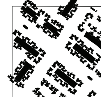
HDB point block Punggol Floor area ratio: 3.6 Average building height: 14 storeys
